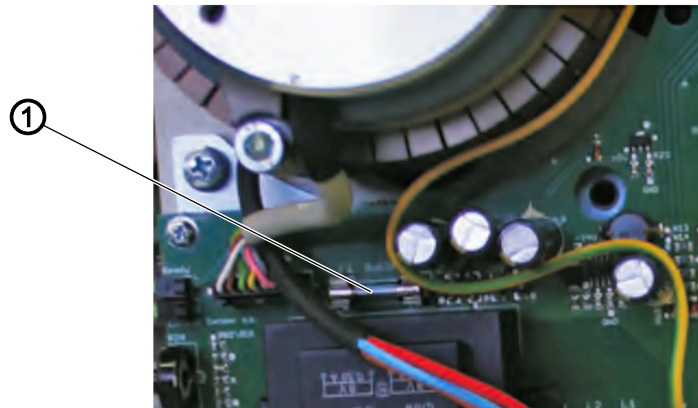
Fig. 85: Replacing the fuse of the sewing light transformer
