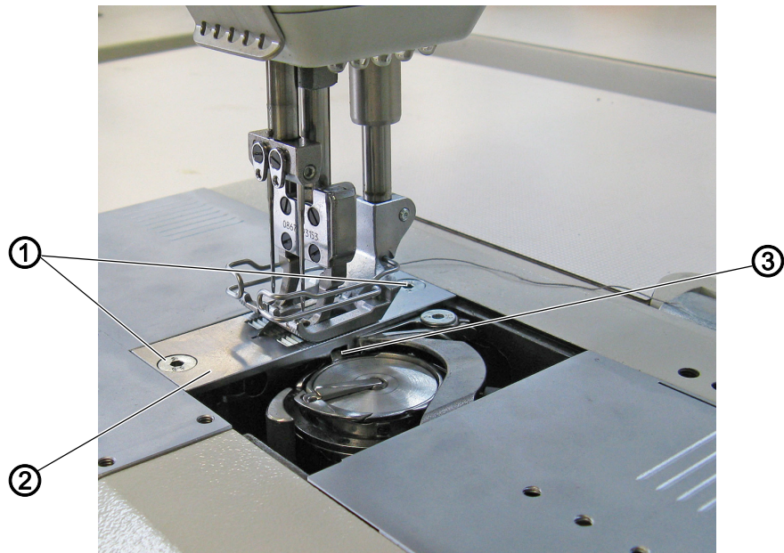
Fig. 6: Assembling and disassembling the throat plate
